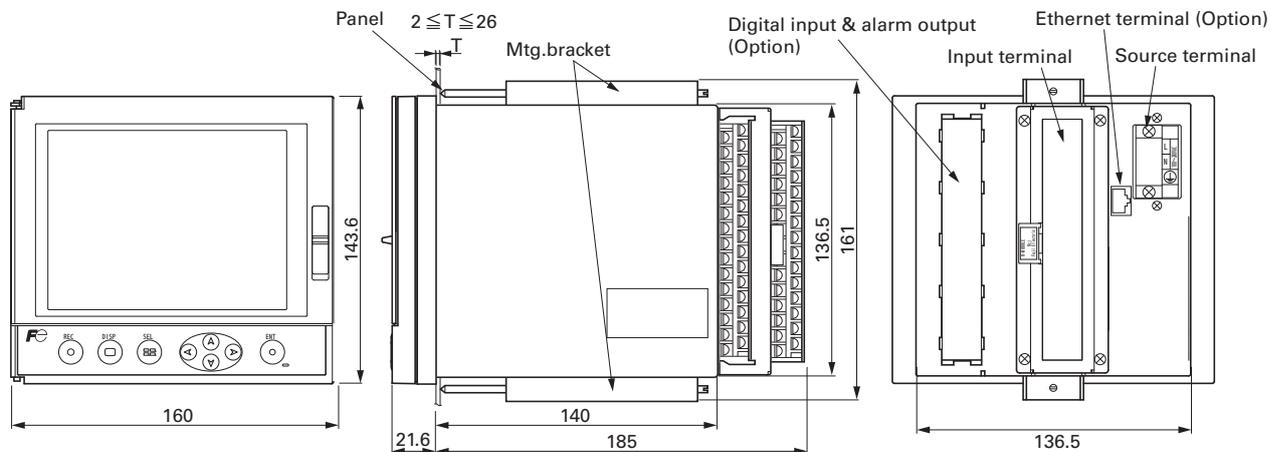
(Note) When placing the main unit on another instrument or on the floor, allow a space of 100mm or more between the unit and instrument or the floor.
