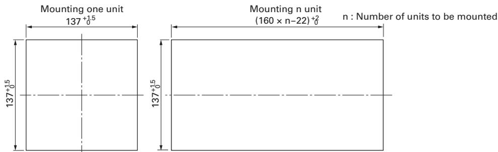
Do not use the water proof packing in case of mounting n unit
