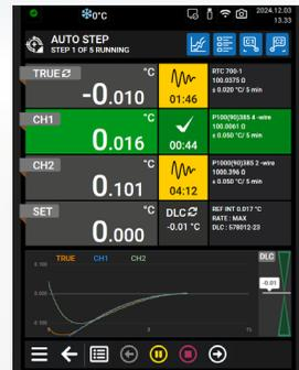
The RTC<sup>t</sup> main screen provides a clear, real-time view of the ongoing calibration with live progress, setpoints, and stability indicators. The patent-pending intuitive graph dynamically adjusts for enhanced precision and deviation detection. Learn more on the [next page](#).
