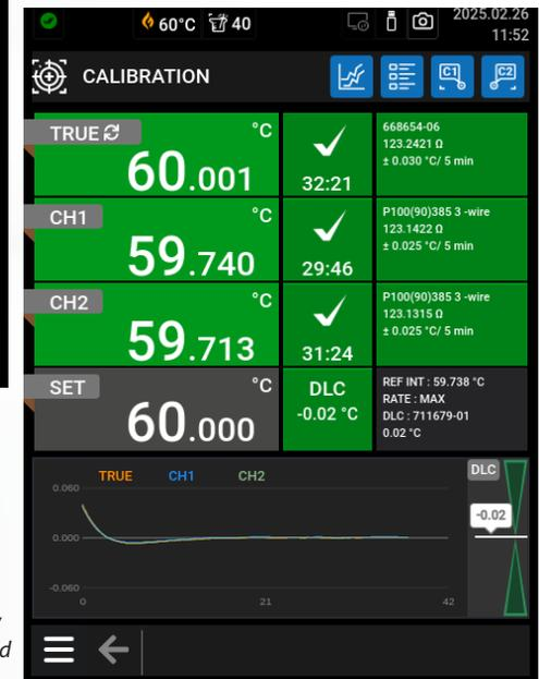
Automatically zooms in on micro-deviations once stability is reached, ensuring unmatched accuracy and confidence.
