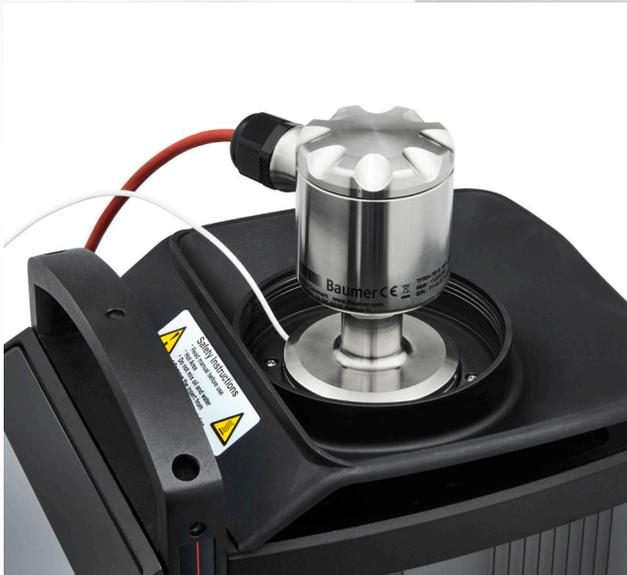
Assembled RTC<sup>t</sup>-156 insert and RTC<sup>t</sup>-168 adapter.
