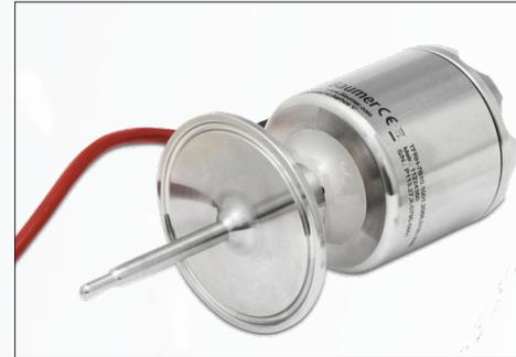
Once mounted, the RTCT-168 combines the external cable reference sensor and the built-in internal reference sensor to fuel its dual-zone technology and proven Set Follows True function to ensure consistent temperature from the main zone through the upper calibration zone. As technicians can easily transport the RTCT-168, they can now provide in-field calibration of difficult sanitary sensors.
