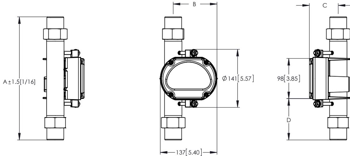
Model 3809 & 3810 General Purpose Indicator Housing with Flanged Connections mm [inches]
