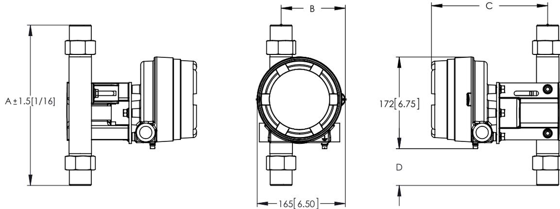
Model 3809 Explosion Proof Indicator Housing with Flanged Connections mm [inches]
