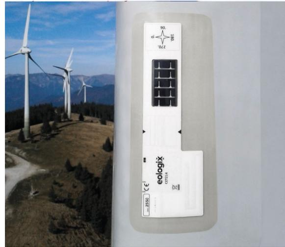
Sensor on the rotor blade
