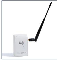
Radio antenna in "USB key" format to communicate with the loggers:
