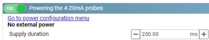
If the external sensor is powered by the logger, then it is possible to use either the internal battery (within the limit of 5 to 18 V and 1.8 Watt maximum) or to connect an external battery between the logger and the sensor. In this case, you need to set up the logger by clicking on the "Go to power management block" link. Setting of the power options is explained in this document in the "External battery and mains power supply" paragraph.
