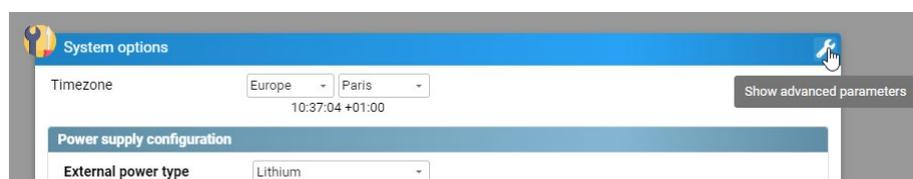
One option in particular appears: "power device from external power". This option is enabled by default.
