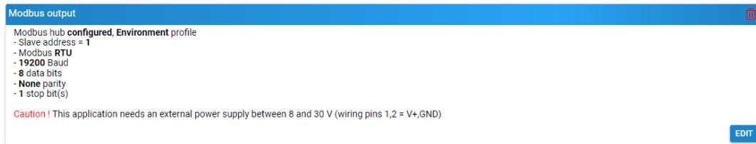
Reminder: the logger must be powered continuously (mains power between 7 and 30V, Lithium battery or lead-acid battery) to allow the Modbus output to function.
