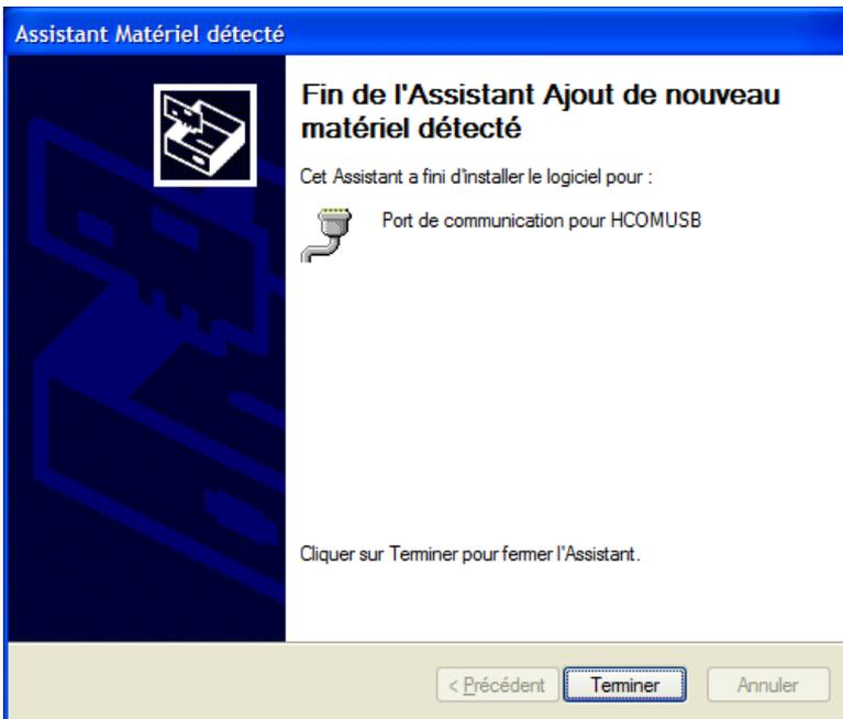
At the end of the installation, a new communication port is added to your system. You can see it using the configuration panel.
