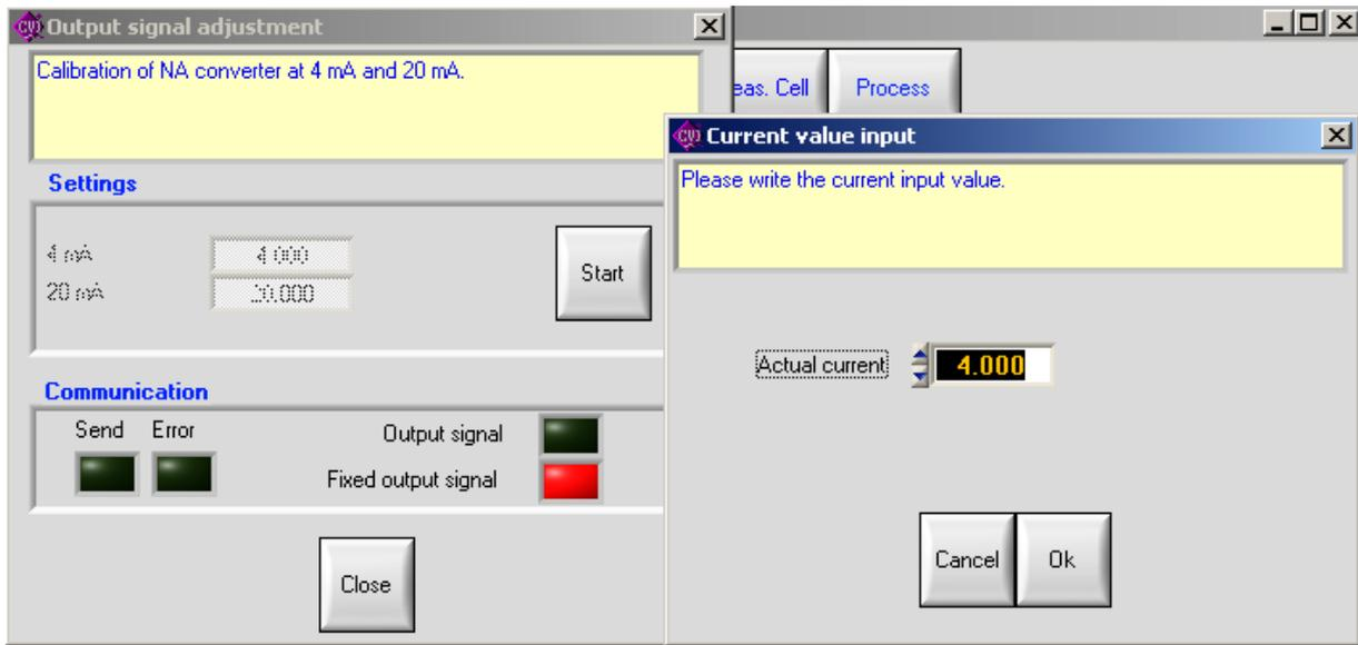
Enter the output signal displayed on the milliamp – meter connected to the transmitter in the “actual current” space.
