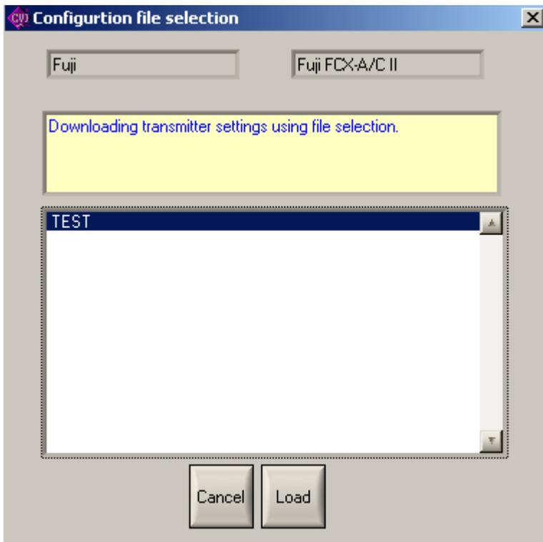
Load an transmitter configuration by clicking on the Load button.
