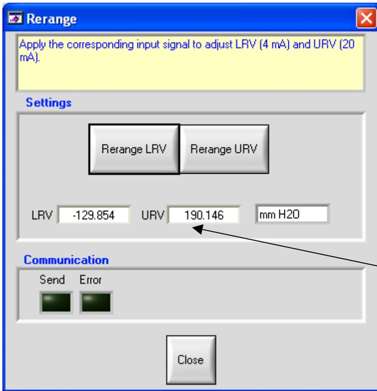
Please mind LRV and URV values showing the zero elevation without changing the transmitter span
