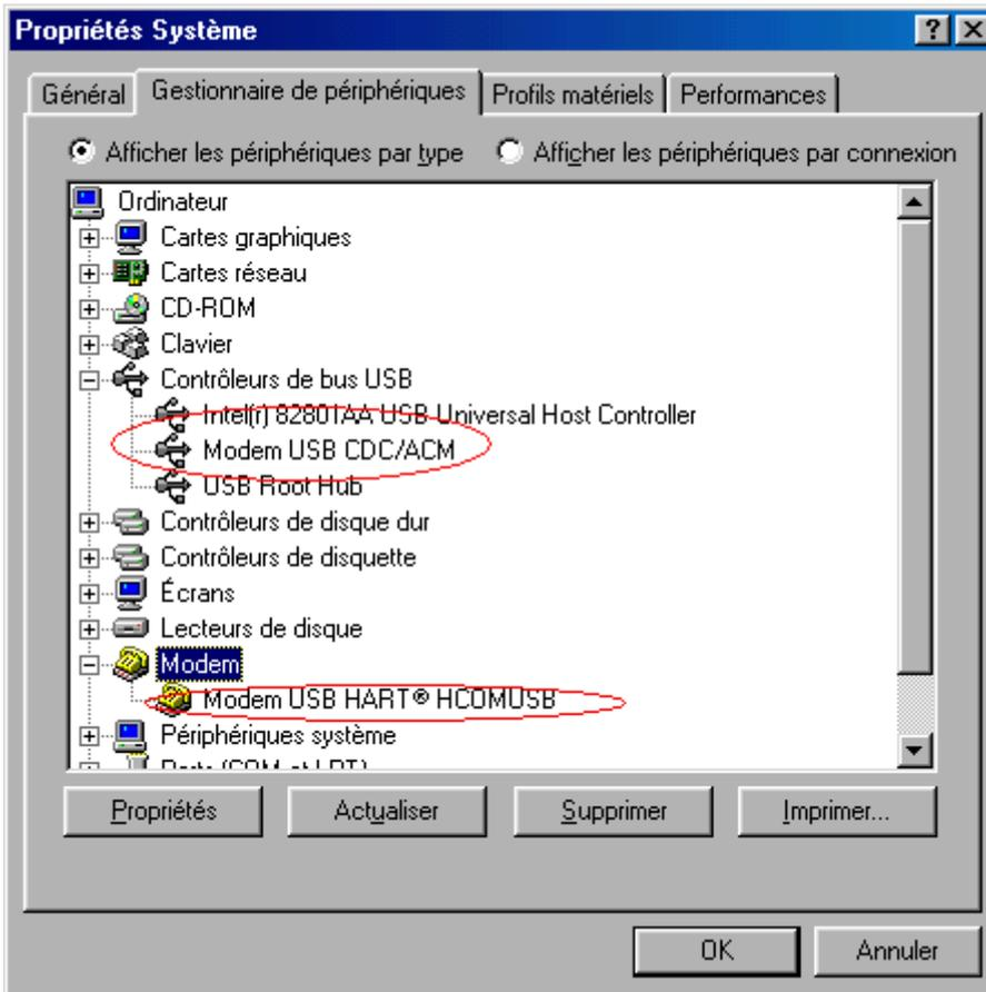
Using the panel configuration >> System icon >> System drivers you can verify that the modem is installed.
